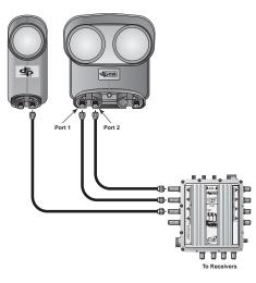
DP Plus Twin & DP Dual connected to a DP Plus 44 Switch
