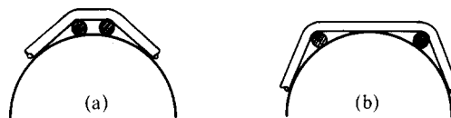
Fig. 10. Effective value of \eta will be smaller in (a) than in (b), since the two nearby cords in (a) share the downward pressure of the upper rope.
